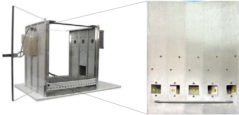
Picture of a 5-CSRTT operant chamber with a food pellet receptacle (left panel), and a curved wall that contains five adjacent nose-poke holes on the right (right panel)
